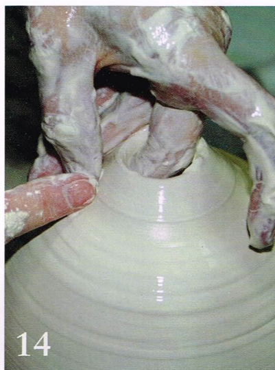
14 Repeat the collaring and thinning process to narrow the top until the opening is the right diameter.
