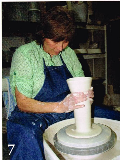
7 Collar the cylinder to regain control if the top becomes off centered.
