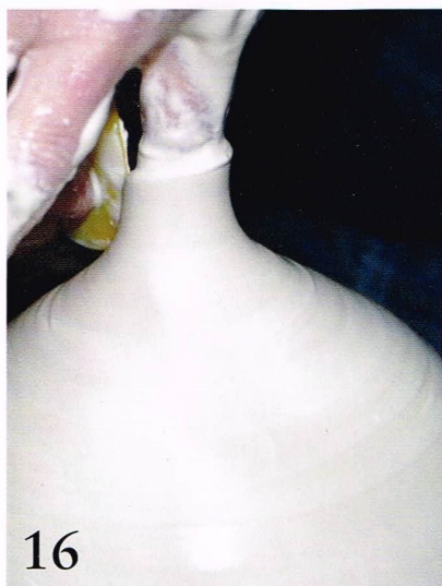
16 Thin the neck using a rib on the outside and a finger supporting the inside.
