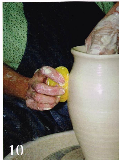
10 Use rubber kidney ribs to remove excess slurry.
