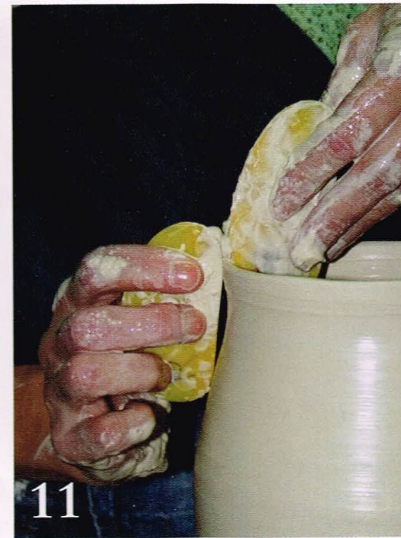
11 Use two rubber ribs to help in the final thinning, or prior to collaring the neck.
