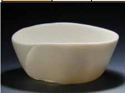
Test bowl #4 with 10% NZK + 15% Grolleg: nice ice white color and good translucency, but needs a stabilizer to prevent slumping.
