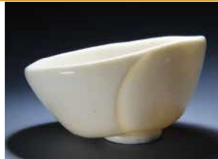
Test bowl #7 with 10% NZK + 15% Tile #6: produced a more stable, white porcelain with less translucency, but more stability in the fire.
